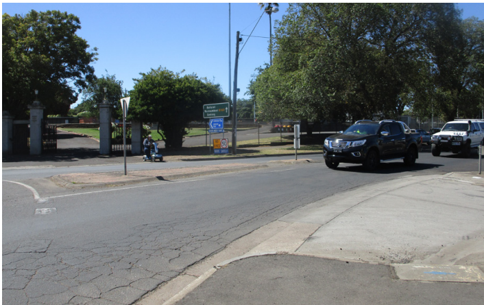
Non-compliant pedestrian crossing from Melville Oval to Thompson St with tactiles located within driveway of service station. Note disability scooter opposite.
