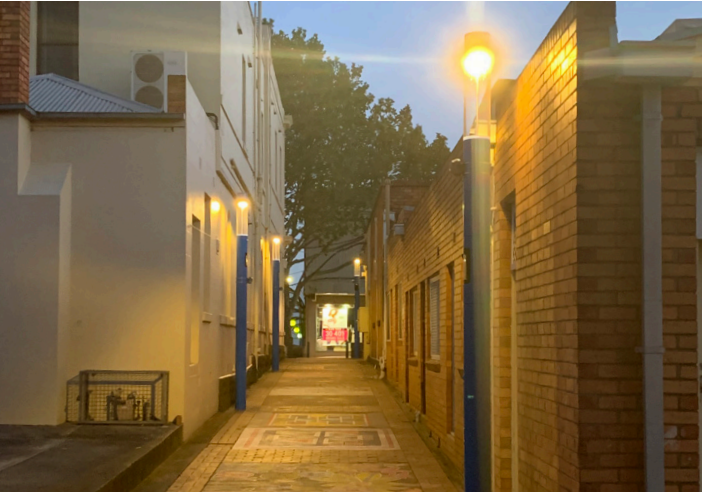
Pedestrian lighting poles with integrated projector technology in McGuigan Lane.
