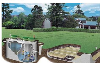
Recirculating sand filter with subsurface irrigation
