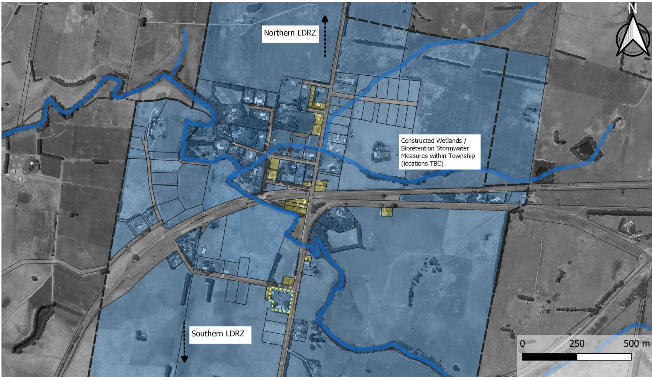
Figure 8: Cudgee Solution Package 2 Servicing Layout - Retain On-site Systems and Build Stormwater Treatment / Detention Measures
