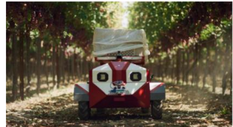
Figure 18: Carry the robot. Can transport 500 pounds of crop and autonomously follows farm workers for a whole day. Pays for itself in 80 days (Nichols, 2021).
