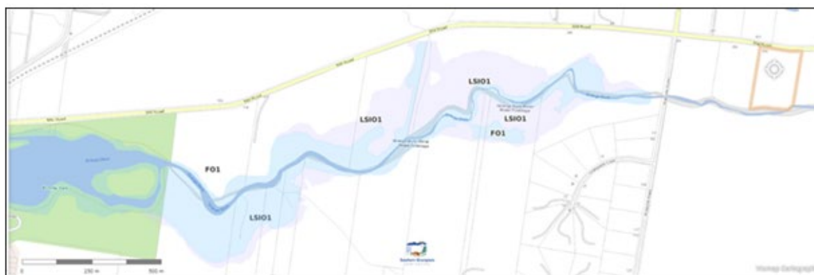
Figure 7: shows the Flood Overlay (FO) and Land Subject to Inundation (LSI01) on and along the Grange Burn to Robsons Road Hamilton where the flood study finishes, up stream of Lake Hamilton.
